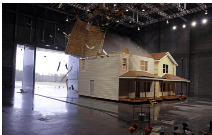
Figure 2: IBHS is one of the research institutes that recreates buildings to test them against high perils side by side and study the differences. Image courtesy of IBHS.org
